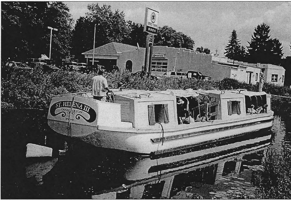
The St. Helena III is a ferro-concrete boat that operates in Canal Fulton, Ohio.
