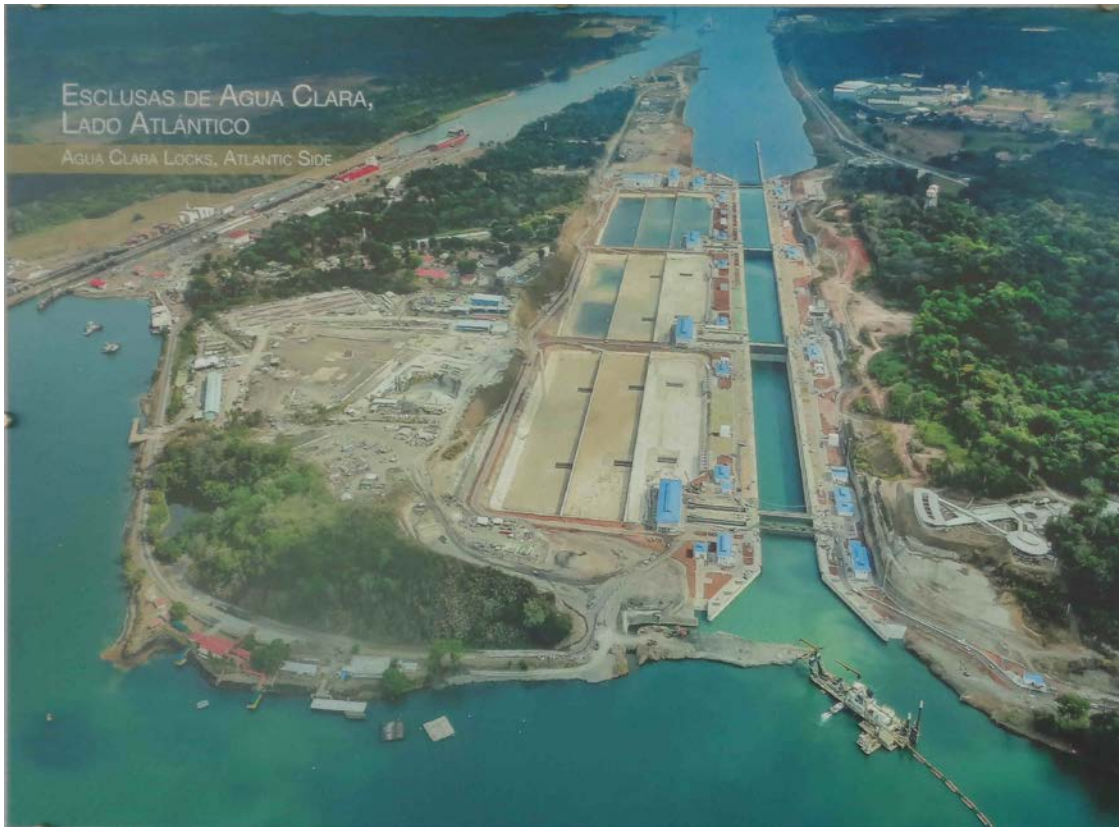
Aerial of new Atlantic end locks looking north with older Gatun Locks on the upper left. Photo was on display at the visitors' center located to the right of the near (in the photo) lock. Three side ponds are visible at each lock.
