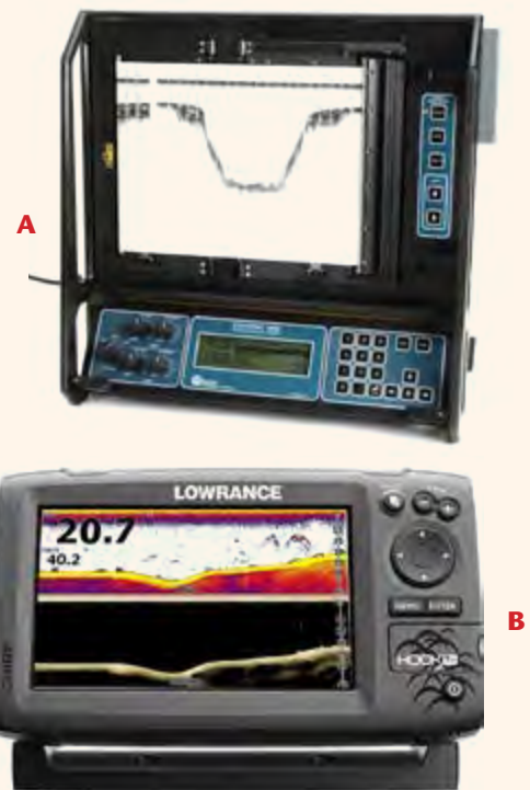
Figure 3. Examples of (A) the older style paper chart echosounders (Odom Mk3) that had no integrated positioning information and (B) the newer PDRs or “fish-finders” of today (Lowrance HOOK-7x) that use GNSS for precise positioning.
