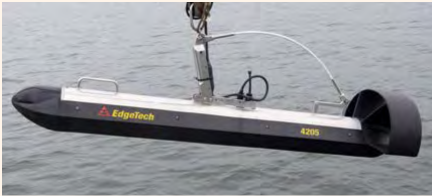
Figure 4. (above) Example of a side-scan sonar (the “fish”) that would be towed behind the vessel and (right) the resulting image is of a shipwreck (not from Seneca Lake). From the EdgeTech 4205 system.
