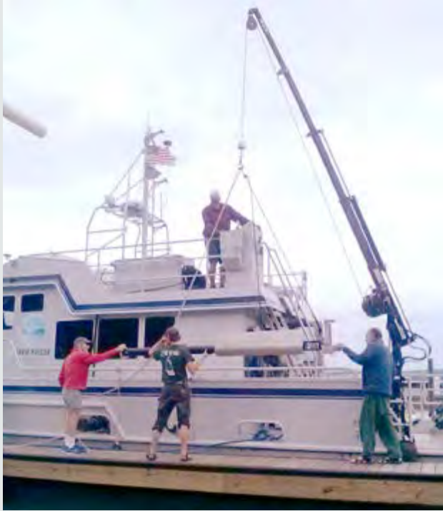
Captain Rich Furbush uses the ship-mounted hydraulic crane to position the multi-beam sonar transducer so it can be secured to the hull. Tom Manley (l) Matt Harrison (c) and Art Cohn (r).
