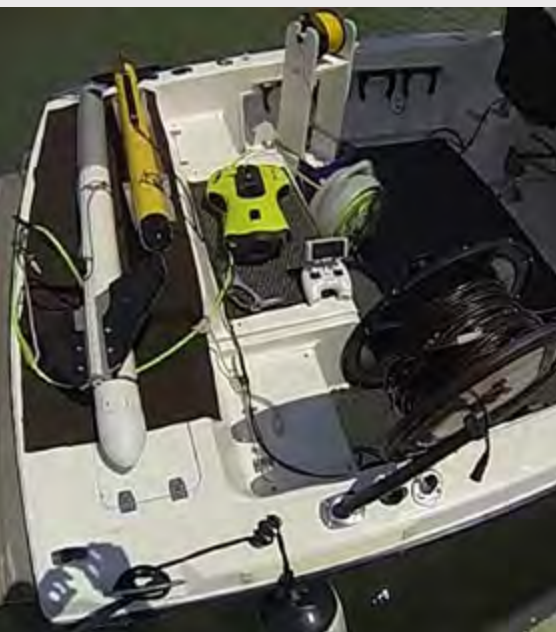
The working end of the Underwater Research Vessel Voyager used on Seneca Lake. It carries both the side-scanning sonar (left) and the ROV systems, which are visible with their associated reels and cables. LCMM
