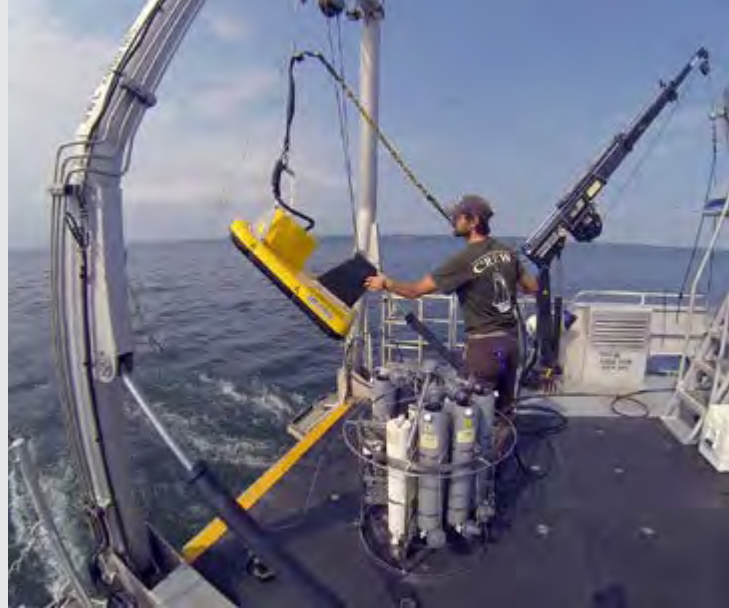
Survey crewman Matt Harrison preparing to deploy the sub-bottom profiler from the stern deck of the R/V Folger . LCMM
