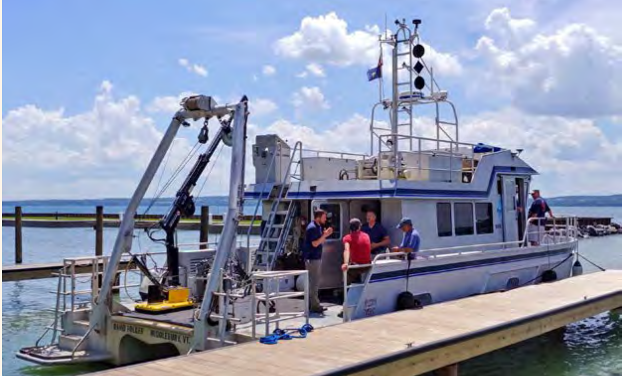
Figure 11. R/V David Folger , the 48-foot, Middlebury College research vessel, was the central platform used in 2019 to systematically survey the underwater bathymetry of Seneca Lake.
