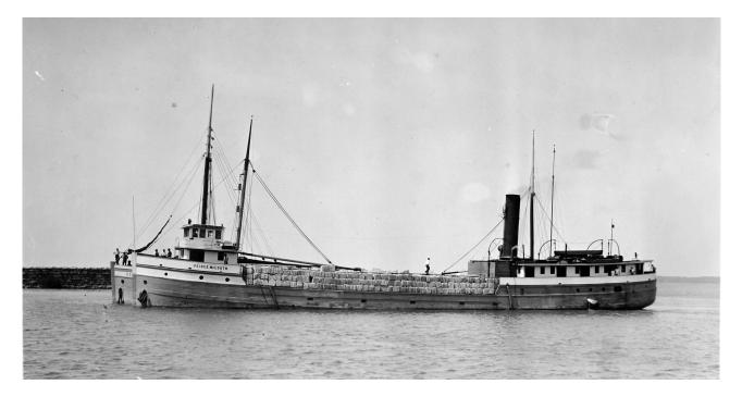
Although these two ships look very different, both had similar capacities in tonnage. The *Peirce McLouth* is shown in the Buffalo harbor in 1921 with a load of wood pulp from Port Arthur on Lake Superior. The *Day Peckinpaugh* was a motorship designed to fit through the New York State Barge Canal. She was the first of her type in the 1920s and is the last surviving example of these ships. Both these ships could carry loads of about 2000 tons.
